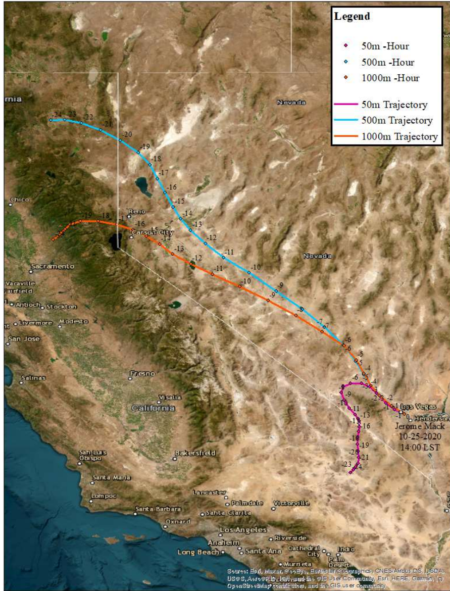
Figure 3.2-1. HYSPLIT 24-hour back trajectories from Jerome Mack on October 25, 2020, at 14:00 PST, originating at (maroon) 50 m, (green) 500 m, and (blue) 1,000 m, with hourly points.
